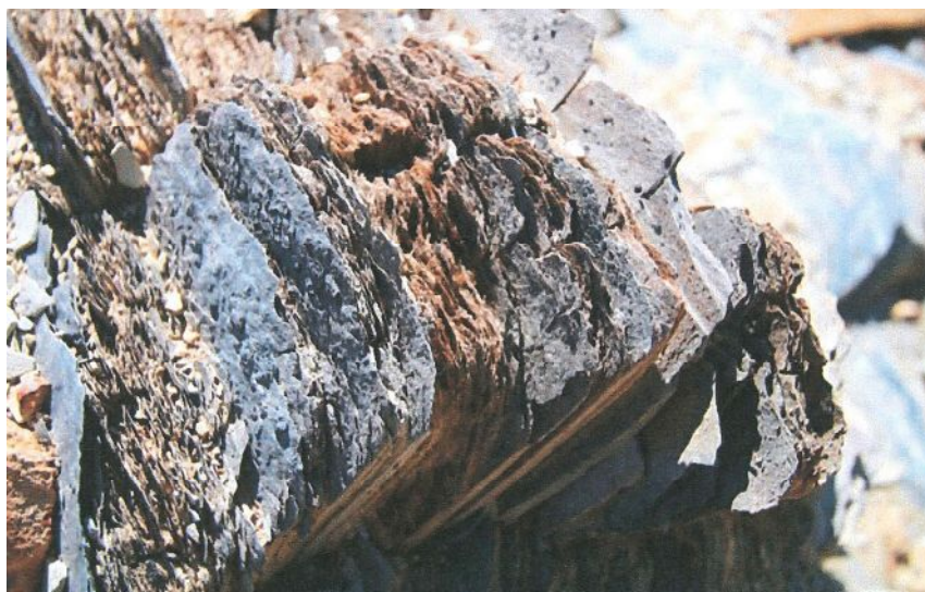
Fig. 3. High-grade oil shale weathered into paper shale, Mahogany Zone, Utah, U.S. The Mahogany Zone contains rich oil shale, averaging up to 80 gallon of oil per ton of rock. From Beckwith R. and Writer S. (2012)
